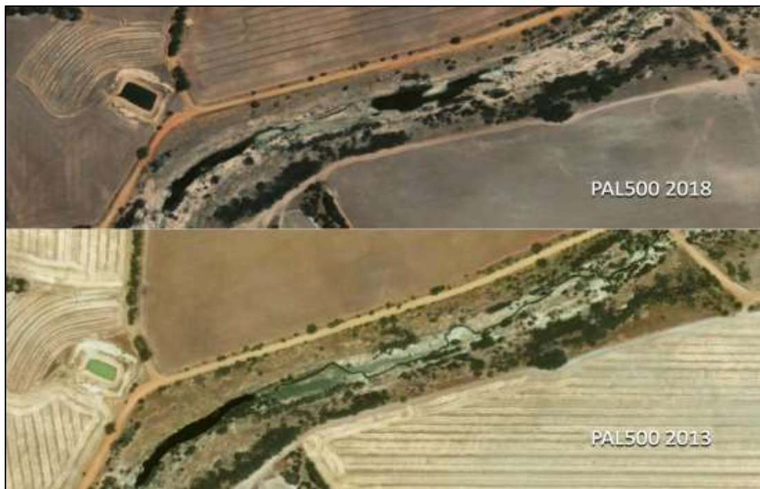
Figure 1: Google Earth imagery showing the movement of large sediment slugs along a lower reach of Warperup Creek in 2018 and 2013.
